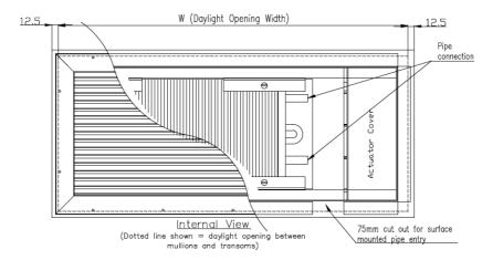
**NOTE:** Heating valve cannot be mounted inside Aircool louvre. Should be mounted upstream on pipe work e.g., above suspended ceiling. Additional support required.
