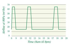
The room becomes occupied and A141PIR senses motion, increasing ventilation to the high rate of 65m<sup>3</sup>/hr for a period of 30 minutes. When the room is unoccupied, and no motion is sensed, the ventilation rate remains at a constant rate of 15m3/hr.
