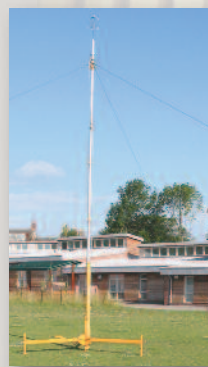
Mast monitoring wind speed and direction at Holymoorside School
