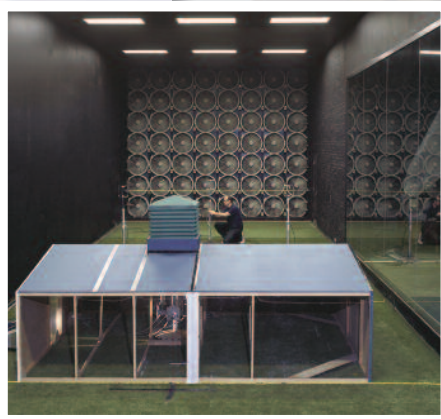
Silsoe Research Institute flow test laboratory measuring airflow performance of Airscoops
