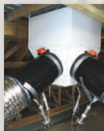
Sonic anemometers monitoring wind flow and direction within an Airscoop
